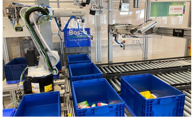
Fig. 1. Robotic bin picking system with six-axis industrial robot, overhead RGB-D camera, tool changer, single-suction gripper, multi-suction gripper, bins containing diverse objects and conveyor belt.
