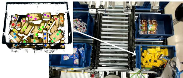
Fig. 9. Visualization of the grasps and corresponding footprints predicted by our approach for an exemplary scene. The executed grasp with selected three-cup footprint is colored in black in the visualization.
