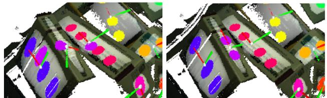
Fig. 6. Example for the edge wrapping issue. For the purple grasp in the left image, a large three-suction cup gripper is incorrectly selected and ignores scene geometry. Instead, a smaller footprint aligned with the object surface would be correct and is the result when applying the proposed method, as shown in the right image.
