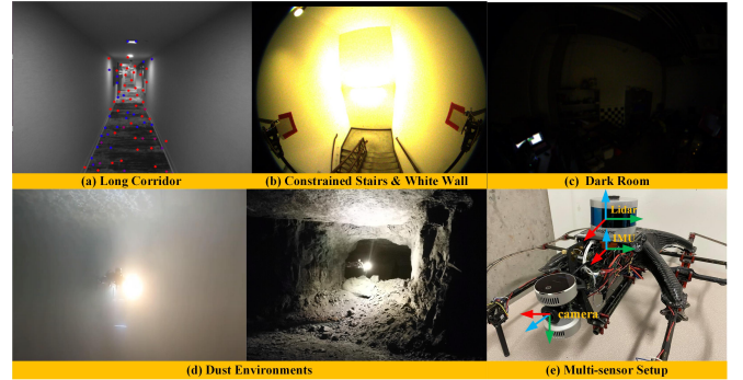
Fig. 4: (a-d) shows the challenging environments where we collect datasets. (e) shows our multi-sensor setup.
