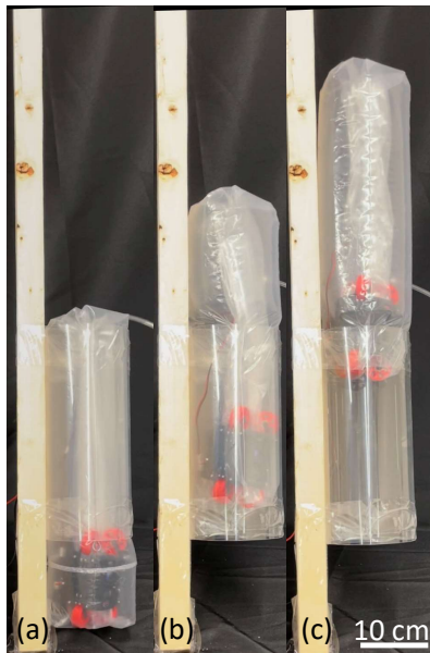
Fig. 8. Demonstration of our soft everting toroidal robot climbing up a vertical pipe. Photos show the view from the side as the robot propels itself upwards, (a) beginning at the initial position at t = 0 s with the propulsion device below the pipe, (b) moving at t = 2.5 s half-way up the pipe, and (c) ending at t = 5 s at the top of the pipe.
