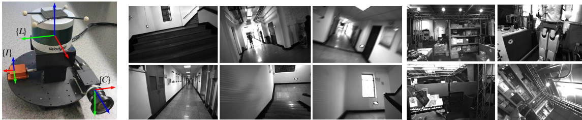
Fig. 4: Left: Sensor suite with a Velodyne VPL-16, Xsens IMU, and a monocular camera. Middle: Snapshots of Teaching Building sequences. Right: Snapshots of Vicon Room sequences.
