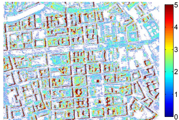
Figure 3. Point density [points/m 2 ] of a test area near Berlin central station.
