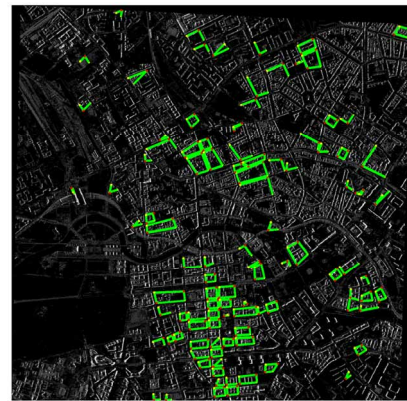
Figure 6. Matched L-shapes, and their end points. Incomplete L-shapes are also allowed, if the same L-shape is detected in both point clouds.
