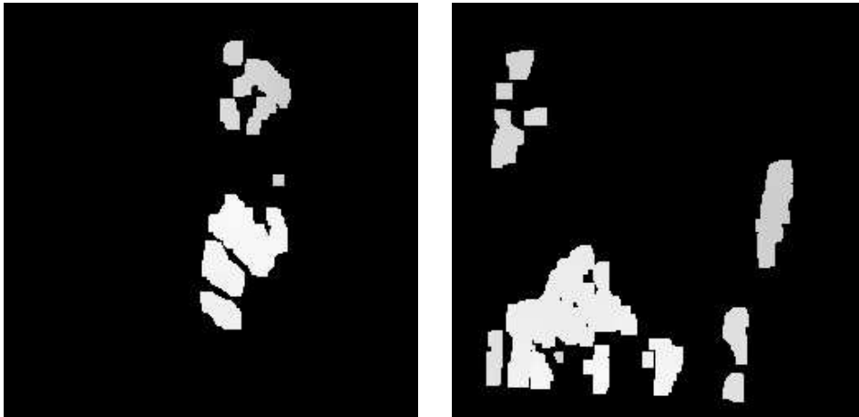
Figure 7: The absolute value of the negative disparities on the left, showing that the fist and a portion of the arm are between the robot and the plane of rectification, and the positive disparities on the right, corresponding to the points located beyond the plane.
