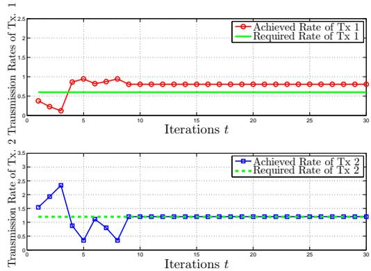
Fig. 2. Instantaneous achieved rates of transmitter 1 (red) and 2 (blue). Average SNR  $\frac{p_{k,\max}}{\sigma_k^2} = 10$  dBs,  $\Gamma = (0.6, 1.2)$  and  $N = 32$ . Channel realizations in Fig. 2 and Fig. 1 are the same.
