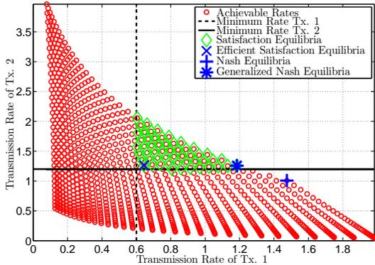
Fig. 1. Achievable rates and equilibria of the 2-transmitter interference channel for a particular channel realization. Average SNR  $\frac{p_{k,\max}}{\sigma_k^2} = 10$  dBs,  $\Gamma = (0.6, 1.2)$  and  $N = 32$ . Channel realizations in Fig. 2 and Fig. 1 are the same.
