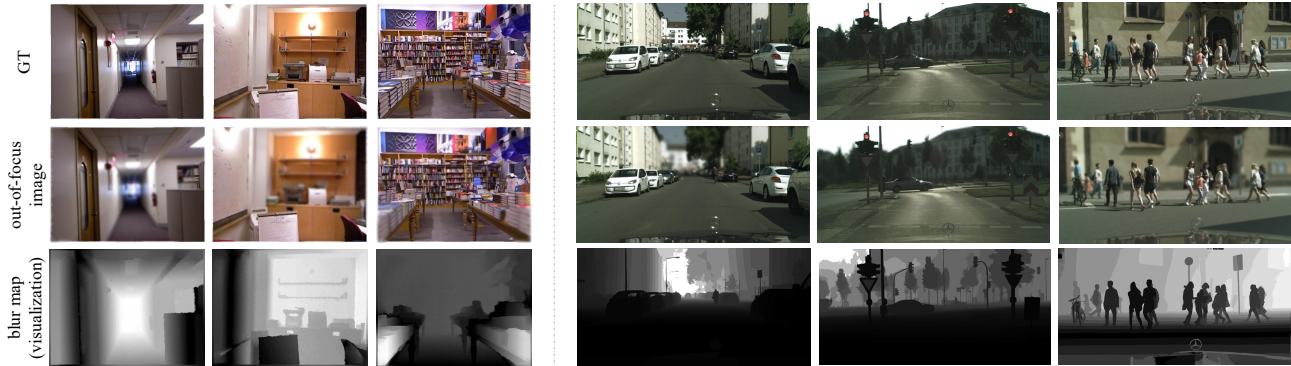
Figure 3. Original RGB images, the generated out-of-focus images and blur maps. The changes from dark to light in blur maps indicate that the corresponding out-of-focus image changes from clear to blur. The first three columns are images from NYUv2-BSR, and the last three columns are images from Cityscapes-BSR.
