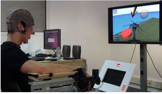
Fig. 5. Experiment in the virtual environment. Here the subject is using the 3D touchless interface with his right hand and the SSVEP LEDs are put in front of him. The screen displays an helicopter in the virtual environment. The subject should pass through all waypoints, materialised by red (or grey) disks on the screen. When the subject triggers a shortcut, the helicopter is moved to a location materialized by the transparent ball.
