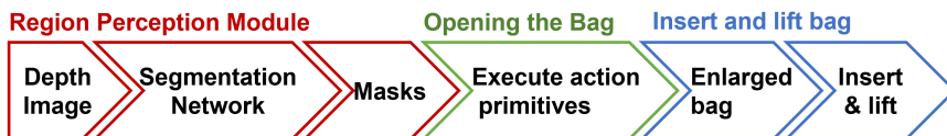
Figure 4. Pipeline for our method: The perception module takes depth images and outputs segmentation masks for the bag handles and rim. The robot grasps the key points and executes dynamic actions. Last, the robot inserts the items and lifts the bag .
