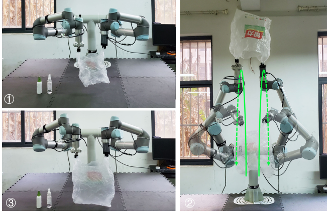
Figure 7. Dual-arm Shaking: ① Preparation for dynamic dual-arm shaking. ② Long-distance and high-speed shaking. ③ An enlarged bag .
