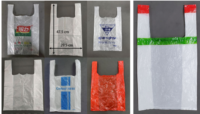
Figure 3. Left: Various plastic bags adopted to train and test the region perception module. The bags include different sizes, patterns, and different colors. Right: A bag with red paint on its handles and green paint around its rim. The paint color can be changed into others according to the pattern color of the bag .
