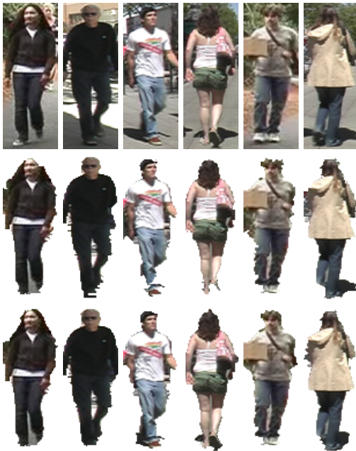
Fig. 6. People silhouette extraction results on the VIPeR dataset (Gong et al., 2014) (line 1 : 6 original images; line 2: the people extraction results obtained with the state-of-the-art scheme of (Migniot et al., 2011); line 3: the people extraction results obtained with our proposed strategy (scheme 3).
