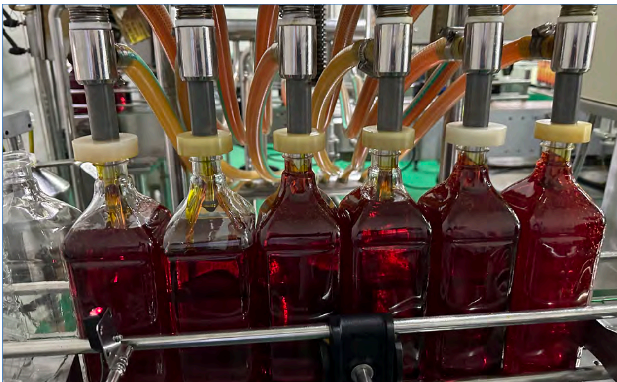
Commitment to quality – Product bottling under stringent hygienic conditions at one of our filling plants at Unitata.
