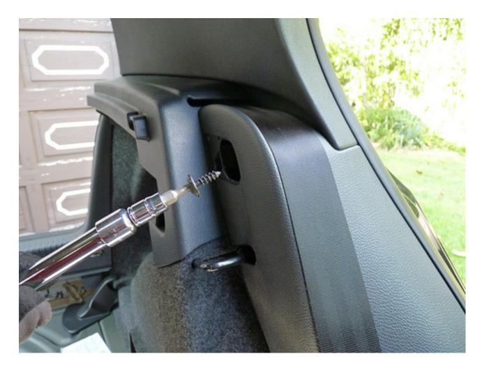
Next locate the 10mm nut on the bottom-circled area. You'll need to remove this as well. Use an open socket wrench or similar unless you have a deep 10mm socket.
