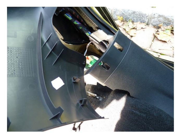
Next go to the rear of the car and open the hatch. Pull the trim material directly next to the tail lights. You don't need to remove the whole thing, just the top portion. It's held in place by 2 metal clips (where the hot dog shaped holes are). If a metal clip gets pulled off the trim and stuck in the hole, use needle nosed pliers to pull off and just slide it back onto the trim.
