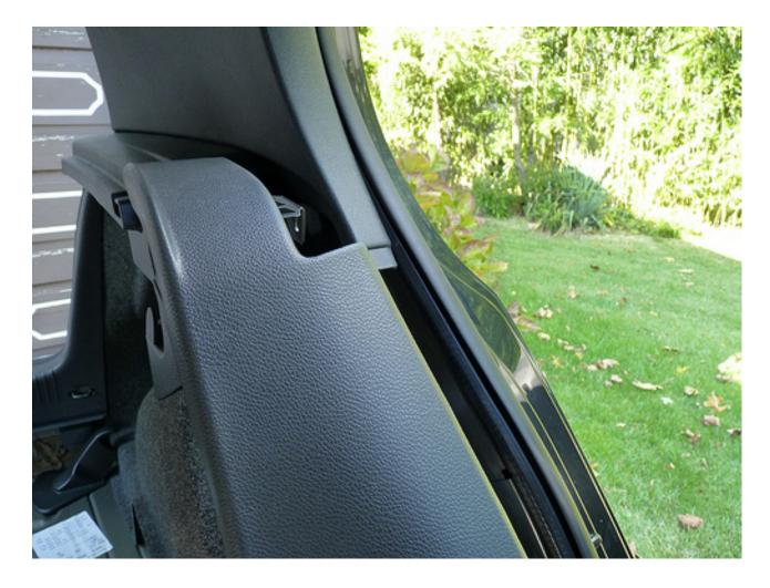
The bottom portion is connected to the lower door trim with two plastic clips. Just pull carefully straight off.
