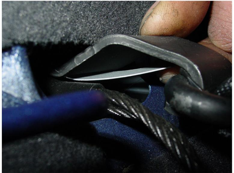
**Step 6 — Remove cargo net anchors**
