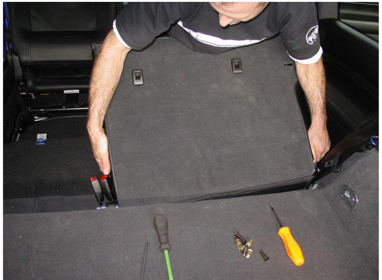
**Step 5 — Unhook middle seatbelt from retainer**
