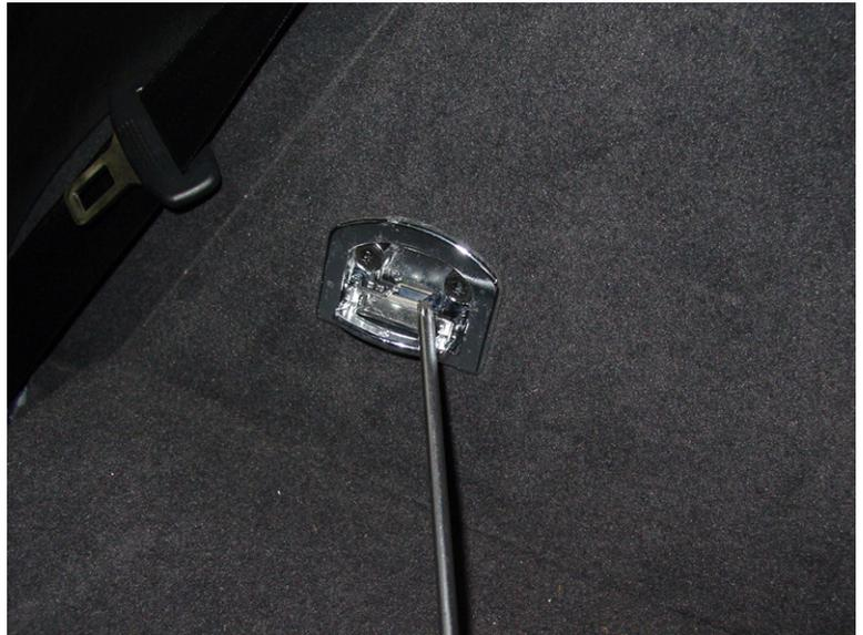
**Step 7 — Locate and remove the interior trim dome fasteners**
