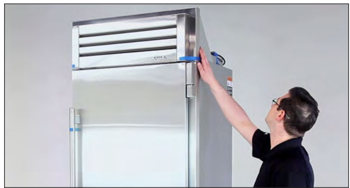
FIG. 2. Inspect the unit's exterior for visible damage.
