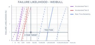
The accelerated tests are composed of heating and cooling cycles, which accelerate battery wear, following the military standard MIL-STD-810. This allows us to simulate longer periods of time – 3+ years, in this case – in a few weeks.
