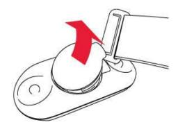
2. Remove the old battery from the battery cover.
