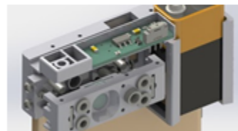
Design concept of the adjustable focusing mechanism
