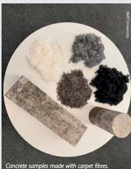
PhD scholar Nayanatara Ruppegoda Gamage and Dr Chamila Gunasekara with concrete samples made using textiles.
