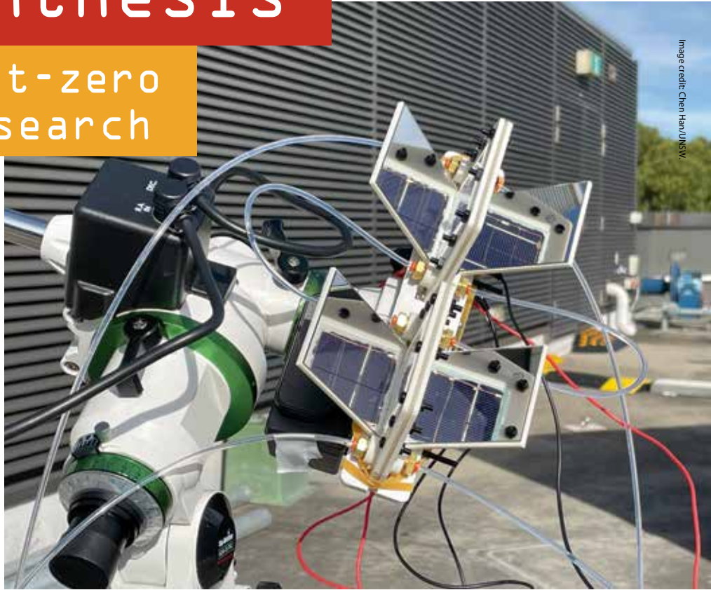
Artificial leaf system developed at UNSW to create ammonia from wastewater using only the sun.
