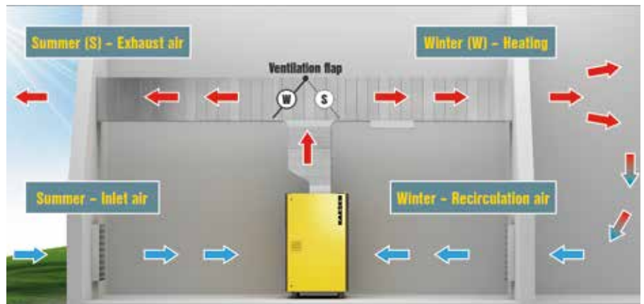
Heated air from the compressor can be used for effective heating of neighbouring spaces via ducting.
