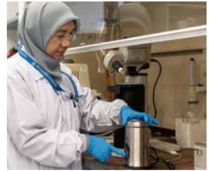
Scrap tyre chips were frozen with liquid nitrogen and ground using a coffee grinder, blended with plastics and placed in a furnace at 600°C. Image courtesy of Monash University.
