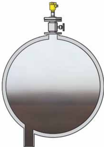
Figure 1: 80 Ghz non-contact radar instruments are useful for level measurement in storage tanks.
