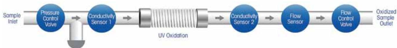
Figure 3: Flow path of a direct conductivity TOC sensor.
