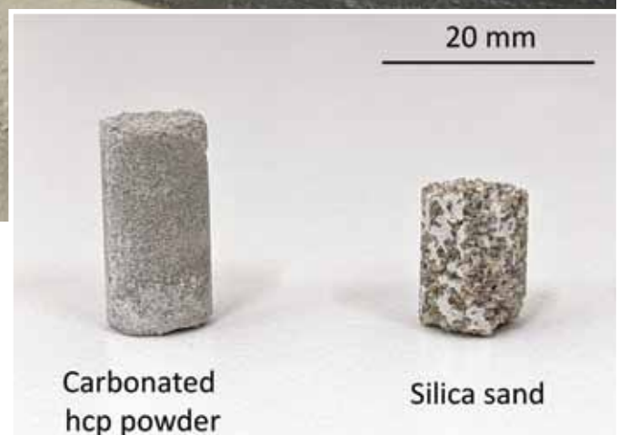
Concrete samples. Two samples of calcium carbonate concrete, one using hardened cement paste (left) and the other using silica sand. Both raw materials are common construction and demolition waste products. © 2021 Maruyama et al.
