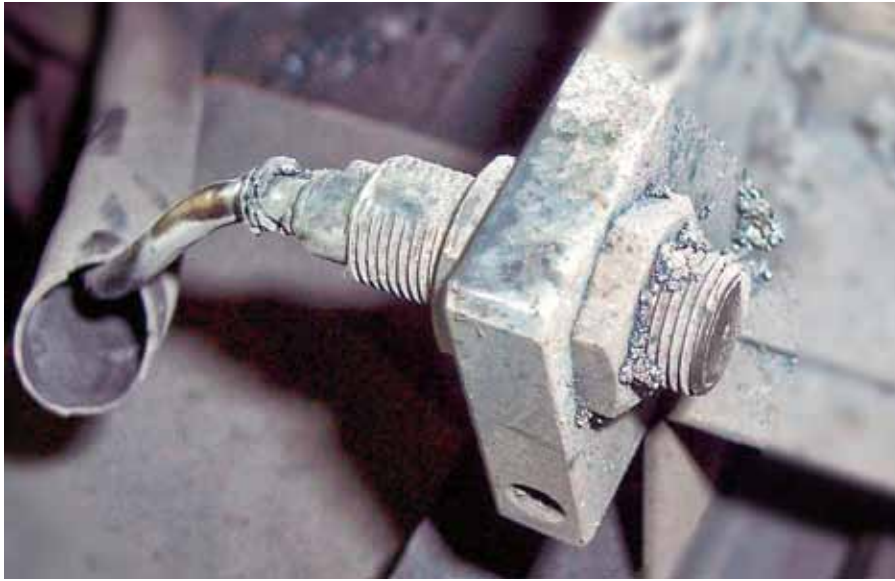
Figure 1: Sensor with weld slag and connector damage.
