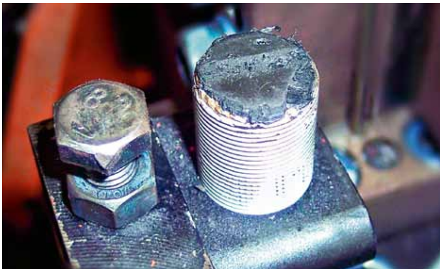
Figure 2: A sensor damaged by impact.
