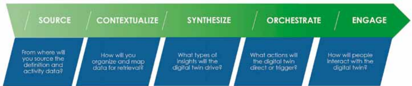
Figure 1: A framework for digital twin development.
