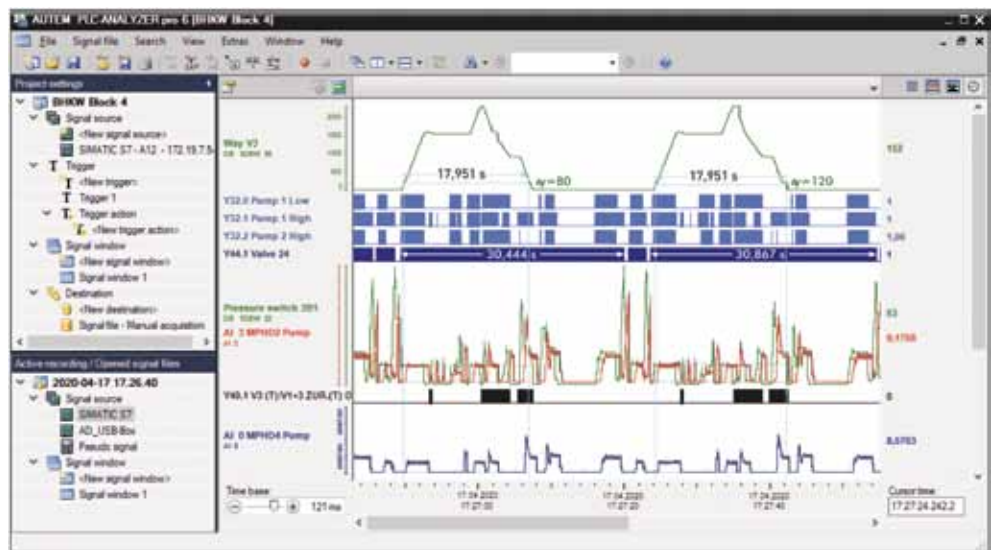
Figure 3: Correlating signals at different locations in the system.
