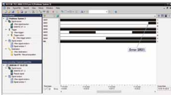
Figure 1: Diagnosis of sporadic faults with PLC-Analyzer.
