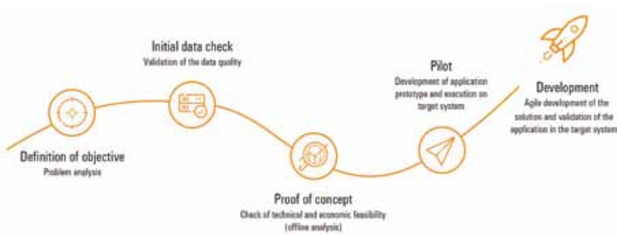
Figure 2: The phases of an industrial analytics project.
