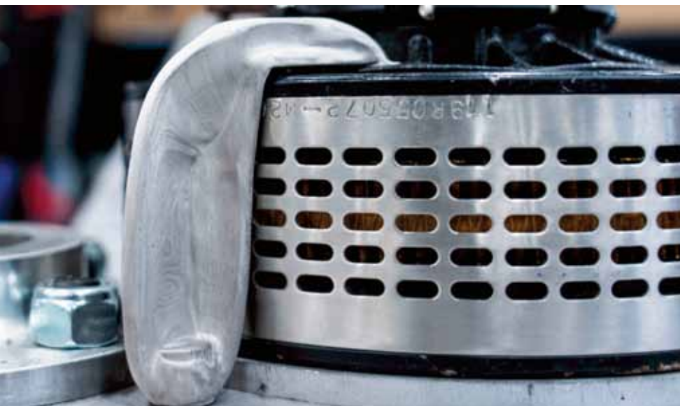
Figure 2: A generatively designed bracket for a heavy-duty robotics application.
