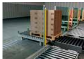
MLC SPG - Safety Light Curtains with Smart Process Gating. Efficient access guarding without muting sensors.
