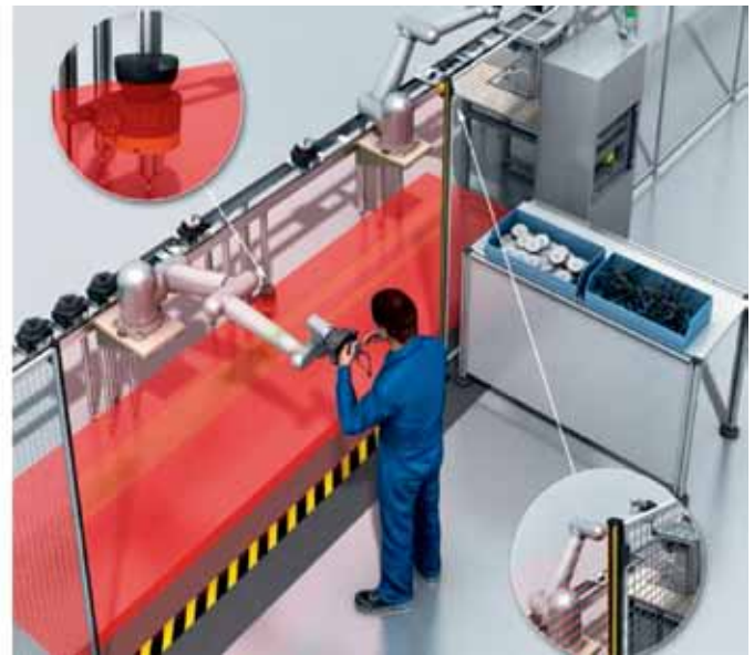
Figure 3: Human and robot collaboration requires the use for force, speed and torque control with robot equipment specifically designed to operate in a collaborative mode.
