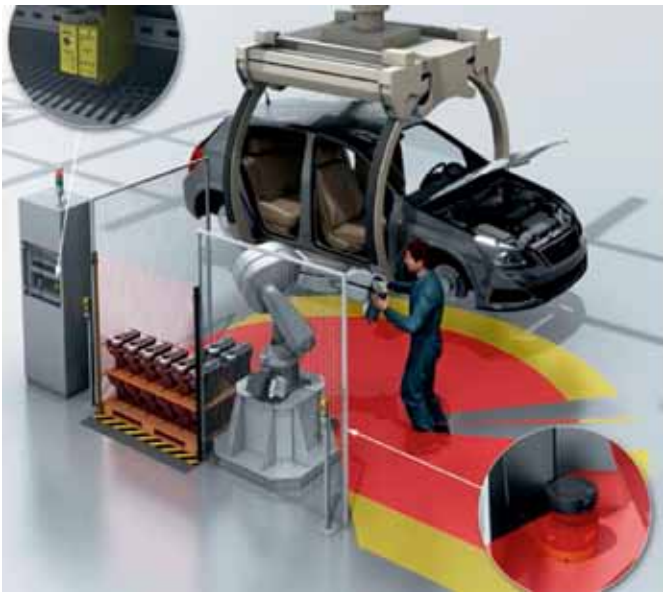
Figure 3: Human and robot collaboration requires the use for force, speed and torque control with robot equipment specifically designed to operate in a collaborative mode.
