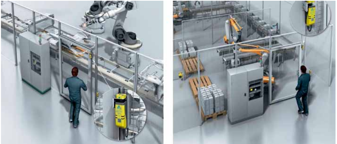
Figure 1: Robot and human coexistence requires the use of safety barriers and interlocks.
