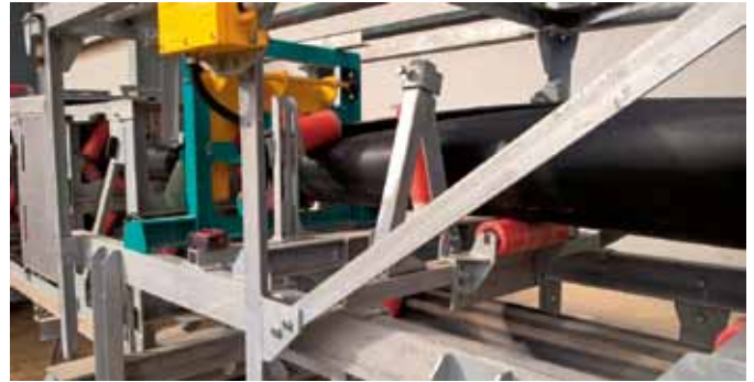
A tube belt conveyor is ideal for containing and transporting light loads.
