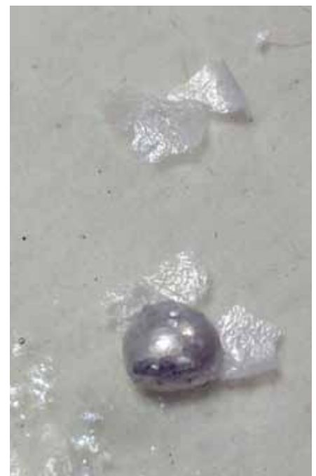
A liquid metal droplet with flakes of aluminium oxide compounds grown on its surface. Each 0.03 mm flake is made up of about 20,000 nanosheets stacked together.
