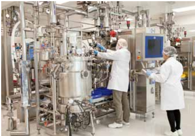
Figure 1: In the life sciences industries, just getting to a temperature sensor can be a problem because of the number of surrounding devices and the need to maintain cleanliness.
