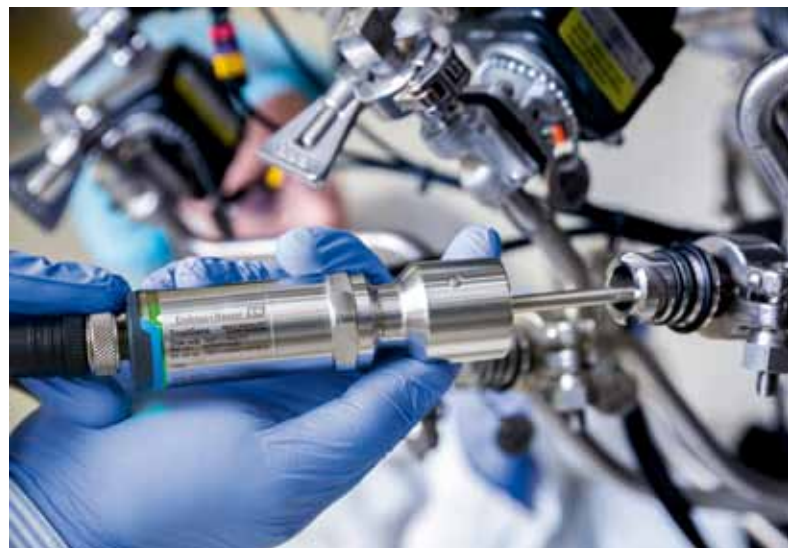
Figure 4: Not having to disconnect wiring from a sensor can cut calibration time in half.
