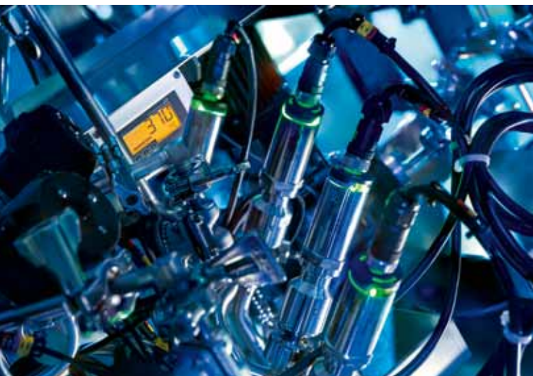
Figure 3: Multiple temperature sensors are used in a fermentation vessel.
