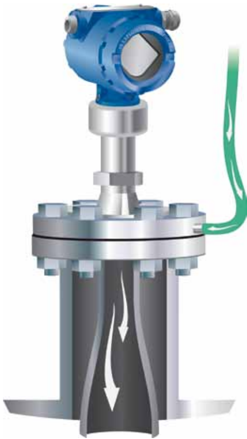
Figure 3: Non-contact radar air purging.
