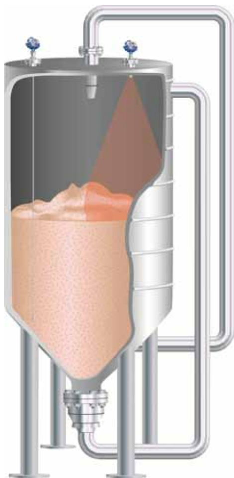
Figure 1: Guided wave radar and non-contacting radar installation.
