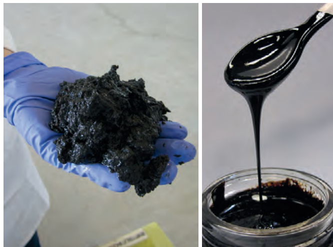
Light: Sludge from Metro Vancouver's wastewater treatment plant has been dewatered prior to conversion to biocrude oil at PNNL. Right: Biocrude oil, produced from wastewater treatment plant sludge, looks and performs virtually like fossil petroleum. Images courtesy of WE&RF.
