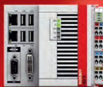
CX5120: Intel® Atom™ CPU, 1.46 GHz, single-core
