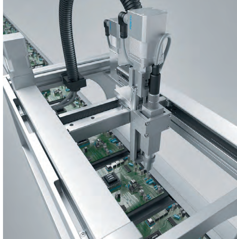
Figure 1: A lightweight gantry robot being used for PCB testing.
