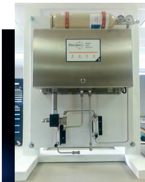
Figure 1: Precise 5 gas analyser – standalone analyser utilising a tunable filter spectroscopy sensor platform (left) and analyser unit with zero/cal sampling system (right).
