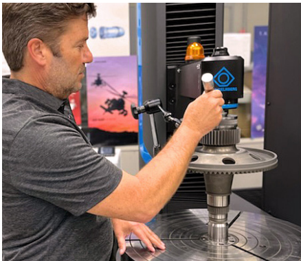
The Klingelberg P65 uses robot-assisted blue-light scanning technology to continually measure within 40 millionths of an inch. These machines communicate directly with our gear grinders.
