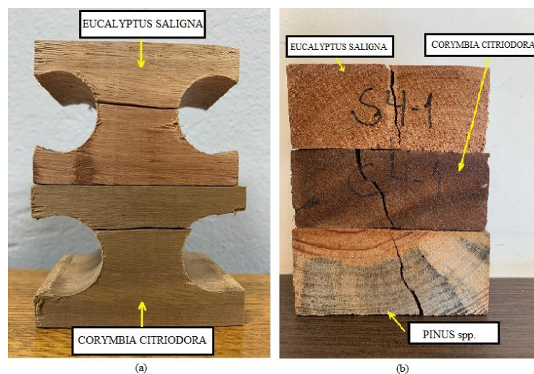
Figure 10. (a) typical failure in specimens submitted the axial test of tensile perpendicular to grain based on ABNT NBR 7190-3 [22]; (b) crack in medullary rays in the specimens from ISO/FDIS 13910 [20].
