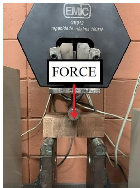
Figure 5. Assembly of the three-point bending test according to ISO 13910 [20].
