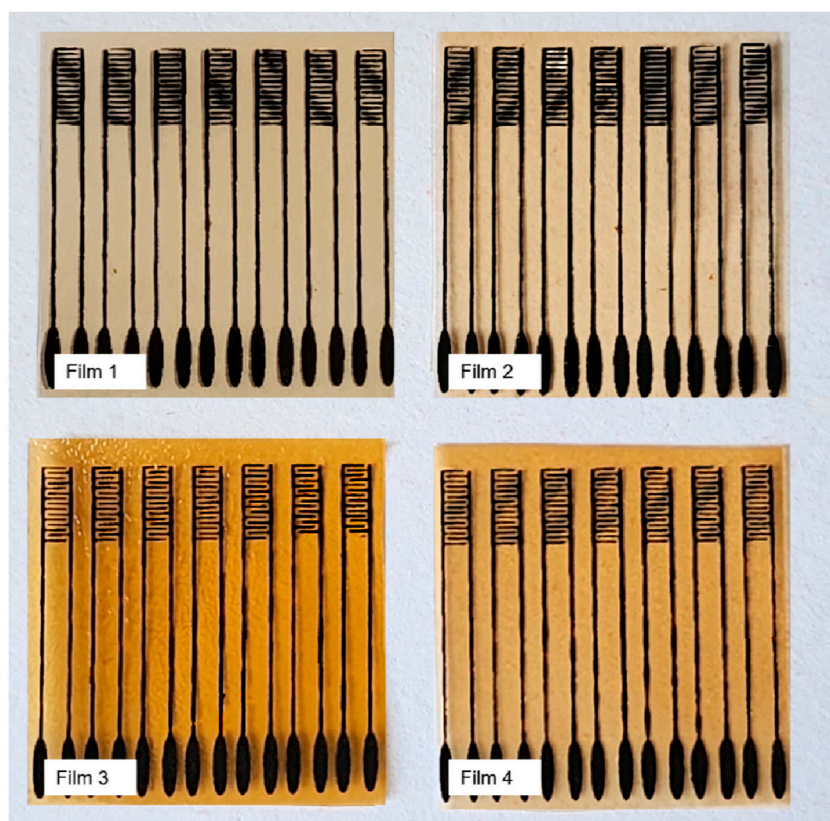
FIGURE 1 Interdigitated electrodes printed on: Film 1: 5% gelatin + 4% tannic acid; Film 2: 5% gelatin + 4% tannic acid + 80°C; Film 3: 5% gelatin + 4% tannic acid + zein and tannic acid coating + 80°C; Film 4: 5% gelatin + 4% tannic acid + zein coating + 80°.
