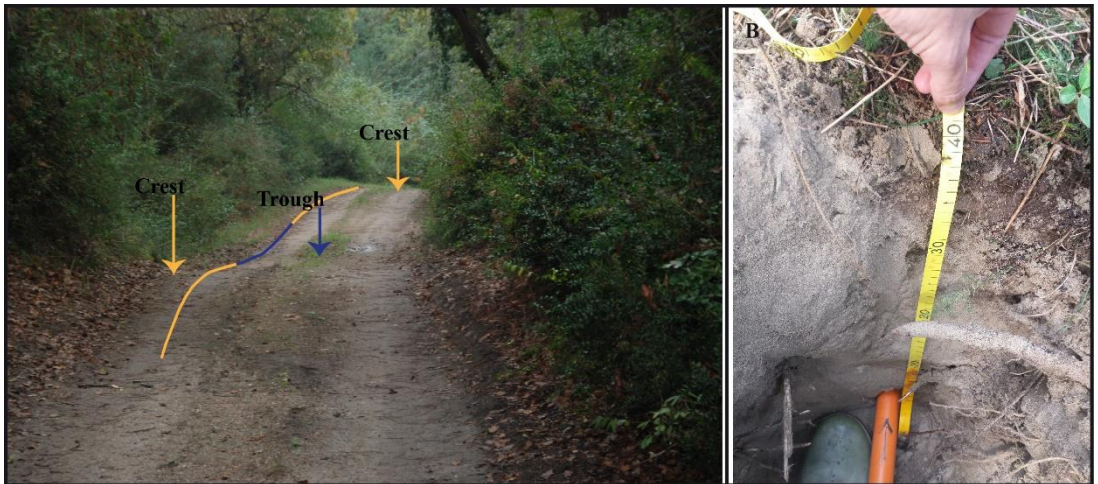
Figure 3. Example of choice of ridges (paleo beach ridges) and trench used in sampling of sediments for OSL dating.
