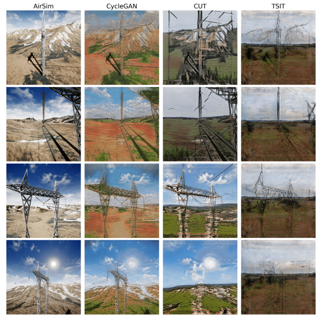
FIGURE 7. Images generated using image-to-image translation. From left to right, the first column represents the original synthetic images provided by the AirSim simulator, followed by the results of the CycleGAN, CUT, and TSIT methods - made by the authors.
