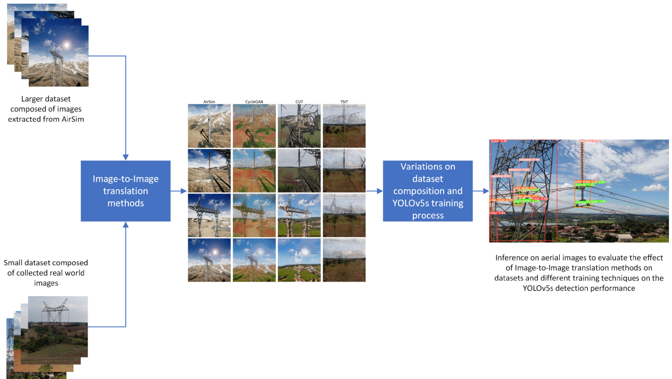
FIGURE 3. Summary of the proposed methodology to study and evaluate methods to improve object detection in aerial inspections of transmission towers within scarce data scenarios. A larger dataset with synthetically generated images and a smaller dataset of collected real images are used to train Image-to-Image translation methods to approximate the simulated environment to the real target environment. Then, variations on dataset composition and training strategies are studied and compared based on the performance metrics achieved by the object detection model on real collected data - made by the authors.
