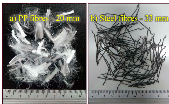
Figure 1. Fiber types: (a) PP fibers; (b) steel fibers.
