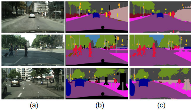
FIGURE 4. DeepLab: (a) Real Image, (b) Results 1 e (c) Conditional Random Field (CRF).
