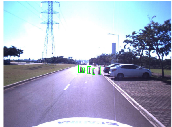
FIGURE 12. Detection of cones in a scene using 3D data - real scene with data provided by stereo vision camera system.
