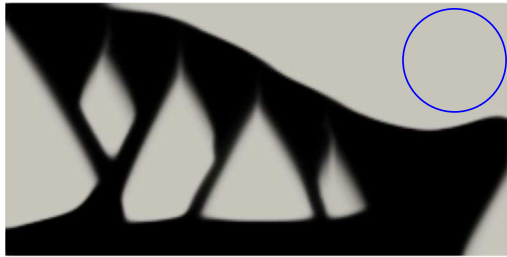
(a) Structure I. Suggested filter radius.
