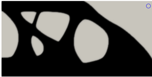
(a) Self-weight-based formulation with w_0 = 0.10 . Compliance of J_D = 73.84 \text{ Nm}
