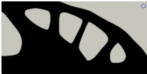
(b) Thermal conductivity-based formulation with w_0 = 0.99 . Compliance J_D = 74.30 \text{ Nm} .
