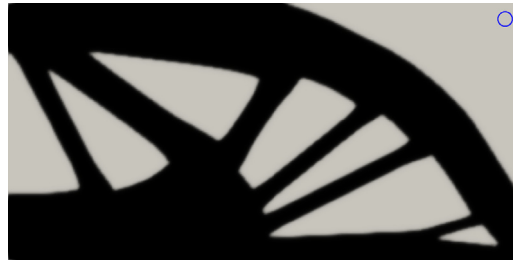
Fig. 19. Standard reference 2D MBB beam design. Compliance J_D = 65.58 \text{ N m} .
