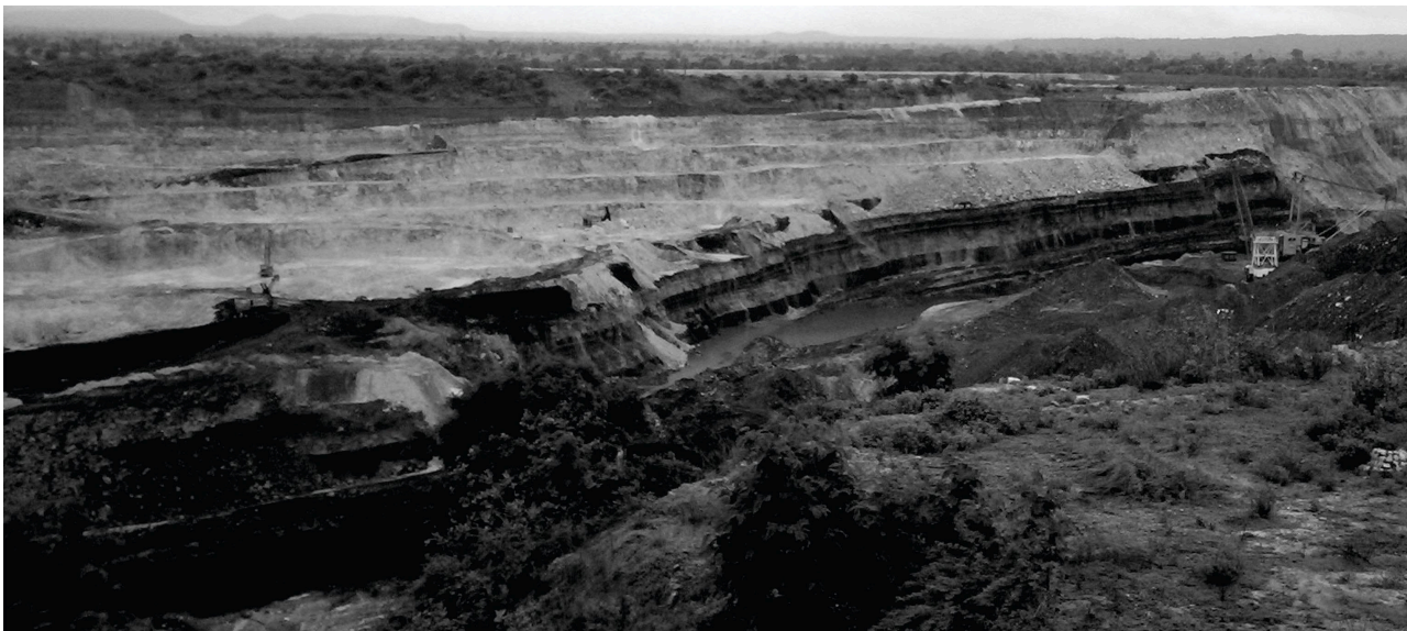
Figure 3. Field photo showing an overview of Bottom, Middle and Top seams with their partings.
