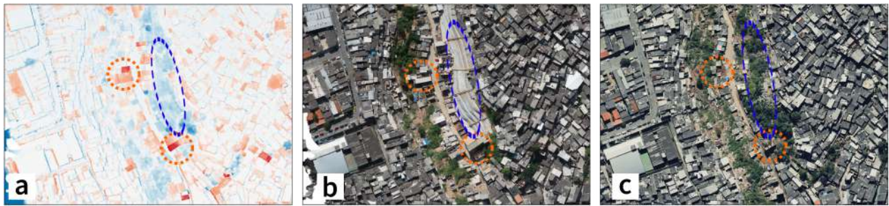
Figure 11. Notable differences with DoD Time 3 for PSM area. (a) DoD Time 3 highlights the increase in the number of floors in buildings (orange circles) and the execution of slope stabilization work (blue ellipse). (b) Orthomosaic of 2022. (c) Orthomosaic of 2017.
