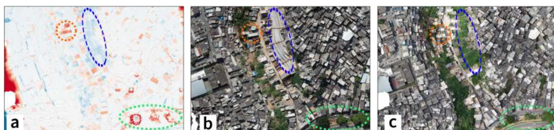
Figure 10. Notable differences with DoD Time 2 for PSM area. (a) DoD Time 2 highlights the increase in the number of floors in buildings (orange circle), the increase in tree canopy size (green ellipse), and the execution of slope containment work (blue ellipse). (b) Orthomosaic of 2022. (c) Orthomosaic of 2019.
