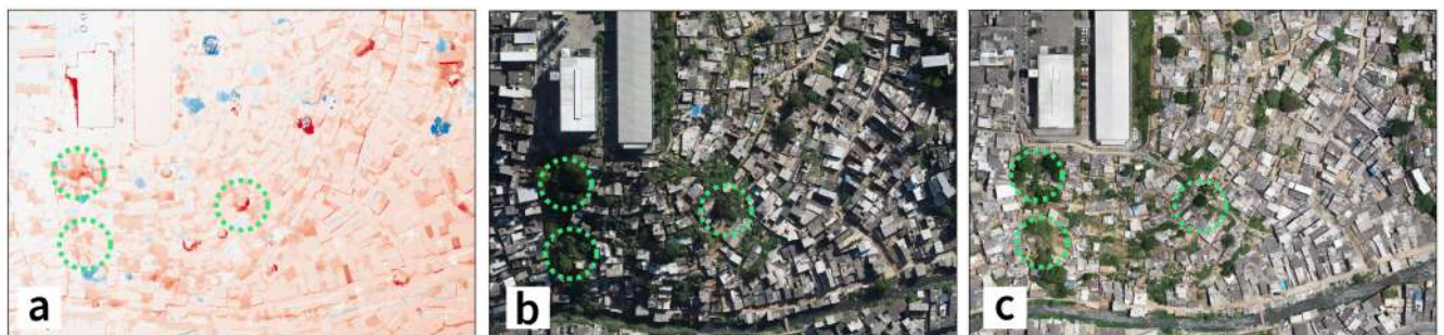
Figure 6. Notable differences with DoD Time 2 for CP area. (a) DoD Time 2 highlights denser settlement and increased vegetation size. (b) Orthomosaic of 2022. (c) Orthomosaic of 2019.
