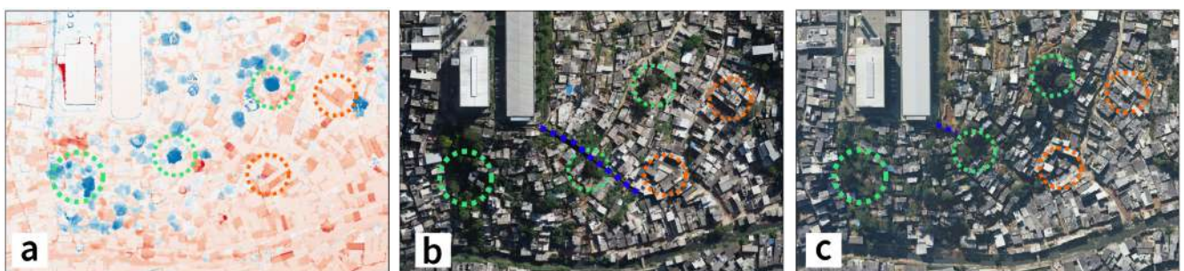
Figure 7. Notable differences with DoD Time 3 for CP area. (a) DoD Time 3 highlights the increase in the number of floors in buildings (orange circles) and the reduction in the vegetation cover (green circles). (b) Orthomosaic of 2022, with the implemented stepped spillway highlighted in blue. (c) Orthomosaic of 2017.
