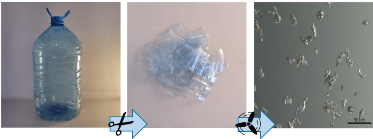
Fig. 1. Process of obtaining and visualizing polyethylene terephthalate (PET) microplastics with a size range of 24 to 32 \mu\text{m} . A) The original bottle of mineral water was obtained commercially. B) Plastic from the bottle cut into approximately 2 \times 2 cm pieces for grinding. C) Visualization of PET particles under stereo microscopy after grinding.
