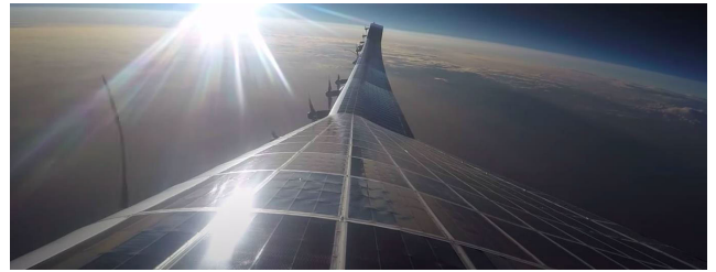
FIGURE 5. “Sunglider” HIBS Platform flying at the stratosphere during an LTE video call communication test between United States and Japan. [Courtesy of HAPSMobile/Loon].
