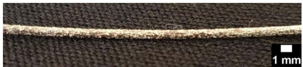
Figure 10. Specimen after 168 h corrosion.
