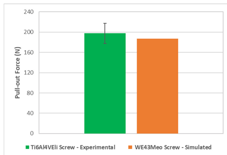
Figure 14. Comparative pull-out strength—experimental results for a screw made of titanium alloy Ti6Al4VEli and the simulated results. In the case of experimental data, n = 5.
