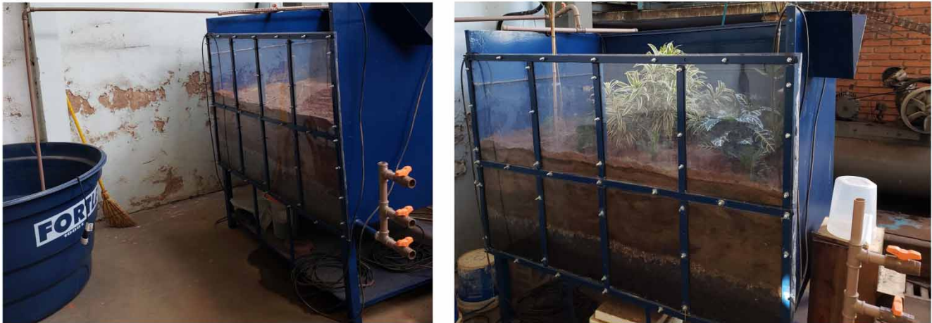
Figure 2 | Bioretention box scheme: the filtering medium is composed of 20% of natural soil and 80% of coarse sand, and drainage medium is formed by medium of medium-sized gravel.
